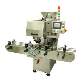
Automatic Multi-Channels Tablets/Capsule Counting Machine TM-406 is designed to feed and count any size, shape or quantity of tablet and capsule (hard shell capsules, and soft gelatin capsules are compatible) with high counting accuracy without change parts. The counting of these products and the indexing of the bottle to be filled is controlled by PLC and Human Machine Interface. It's simple to operate and easy to clean.
